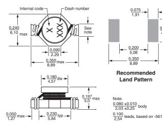
Dimensions are in  $\frac{\text{inches}}{\text{mm}}$
